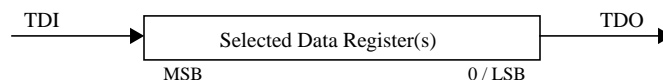
Figure 7.4 TDI to TDO Path for Selected Data Register(s) when in Shift-DR State
